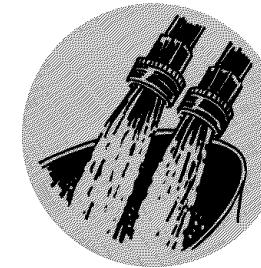
Run water into bucket to determine which hose is hot and which is cold.
