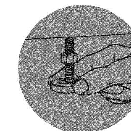
Push on the upper front panel to be sure that the washer is on the rear feet. Lower right front foot to floor. By hand, firmly rotate foot up to an additional  $\frac{1}{2}$  turns. Rock washer gently front to back, side to side and diagonally to check that all four feet are in firm contact with the floor.
