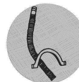
Retrieve hose from parts bag. Feed drain hose into one end of form.
