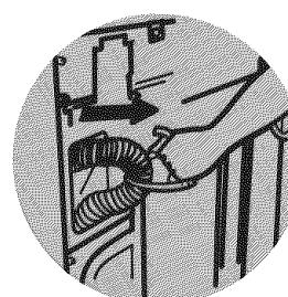
Locate the pull tie to remove drain hose from washer. Pull drain hose straight out of washer from top of hose.
