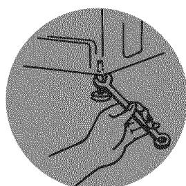
If level, use  $\frac{1}{2}$ " or 14 mm open-end wrench to tighten locknut to washer base.
