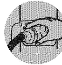
Hand tighten couplings – hot to hot, cold to cold.
