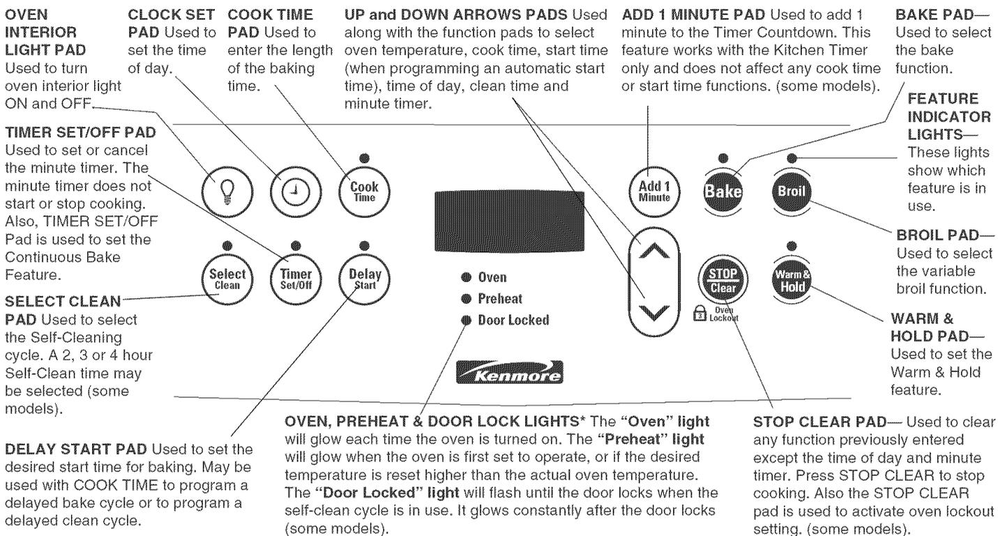
**\*Note:** The **OVEN** indicator light on the electronic display will turn ON and OFF when using the Bake feature and during preheat. This is normal and indicates that the oven is cycling to maintain the selected baking temperature. When preheat indicator light turns OFF, your oven is ready.
