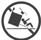
To reduce the risk of tipping, the wall oven must be secured by properly installed mounting bracket provided with the wall oven. Refer to the Installation Instructions for proper mounting bracket installation.
