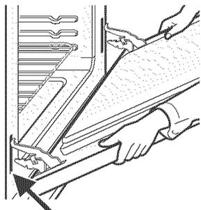
HINGE SLOT - Door removed
