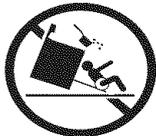
To reduce the risk of tipping, the wall oven must be secured by properly installed anti-tip bracket provided with the wall oven. Refer to the Installation Instructions for proper anti-tip bracket installation.
