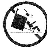
**⚠ WARNING** To reduce the risk of tipping, the range must be secured by properly installed anti-tip bracket(s) provided with the range. To check if the bracket(s) is installed properly, remove the lower panel or storage drawer and verify that the anti-tip bracket(s) is engaged. Refer to the Installation Instructions for proper anti-tip bracket(s) installation.
