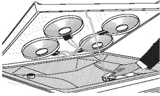
A rod swings up to support the top for cleaning underneath.
