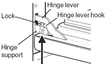
Lock engaged for door removal
