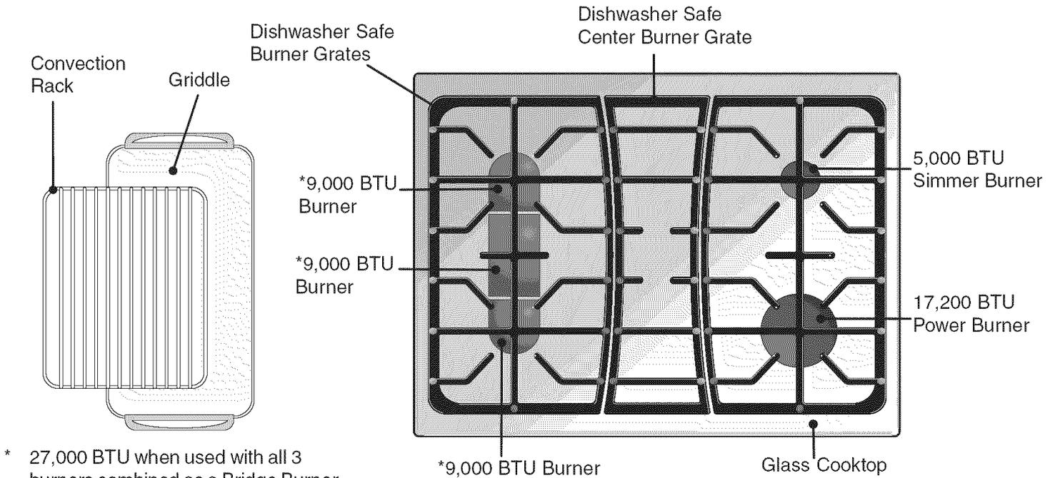
\* 27,000 BTU when used with all 3 burners combined as a Bridge Burner.
