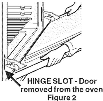
HINGE SLOT - Door removed from the oven
