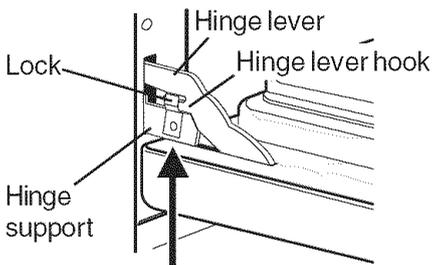
Lock engaged for door removal
