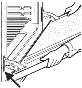
HINGE SLOT - Door removed
