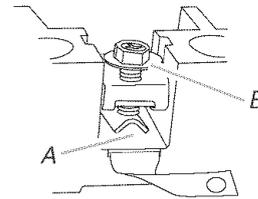
A. Insert wire under screw clamp.
