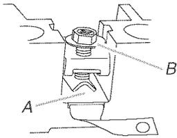
A. Insert wire under screw clamp.
