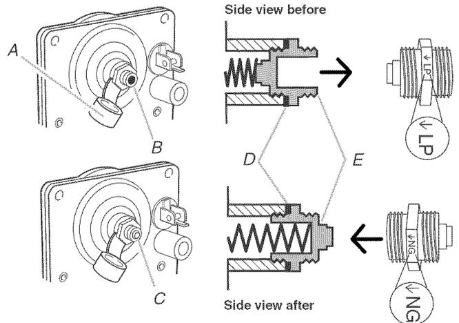
5. Turn over the gas pressure regulator cap and reinstall on regulator so that the solid end faces out and the marking "<- N" is facing the direction shown in the above drawing.
