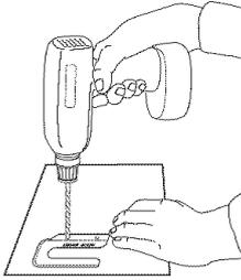
To mount anti-tip bracket to concrete or ceramic floor, use a 3/16" (4.8 mm) masonry drill bit to drill 2 holes at the positions marked on the bracket template. Remove template from floor.
