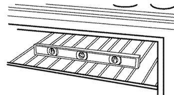
If range is not level, pull range forward until rear leveling leg is removed from the anti-tip bracket. Use 3/8" drive ratchet and channel lock pliers to adjust leveling legs up or down until range is level. Push range back into position. Check that rear leveling leg is engaged in anti-tip bracket.
