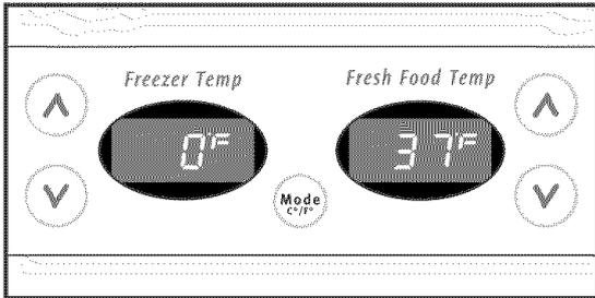
To adjust the temperature to a higher or lower setting, press the **Up (Cold)** or **Down (Colder)** button closest to the display. The first time you press the button, the display shows current setting you entered. Each press of the button after that changes the setting by one.
