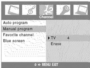
4. Press ▼, and then press ◀ or ▶ to select Memory (add) or Erase. The current channel is added to Memory or erased from the channel list.
