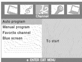
3. Press ENTER to start auto-programming. The TV will automatically cycle through all the TV and Cable channels, and store all active channels in the channel memory.
