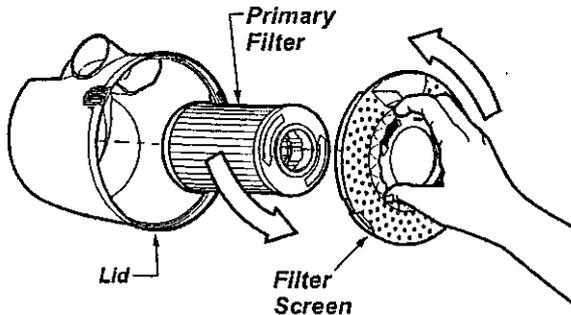
Grasp primary filter, rotate counter-clockwise and lift out. Clean primary filter by gently tapping over a trash container.
