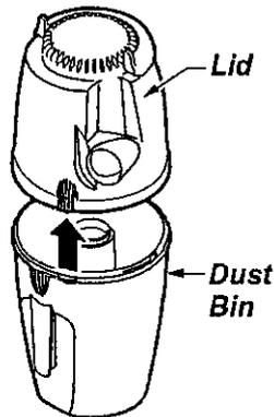
Separate the lid from the dust bin by lifting it straight off.
