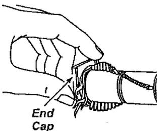
Cut off any carpet pile, hair or lint entangled around the agitator and remove any string or debris located near the end caps.
