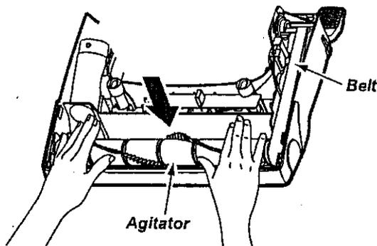
Check to see that the belt is centered on the belt pulley and that the agitator turns freely.
