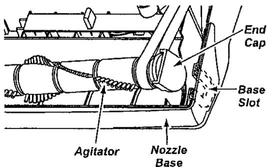
Press firmly, checking to see that each end is completely inserted.
