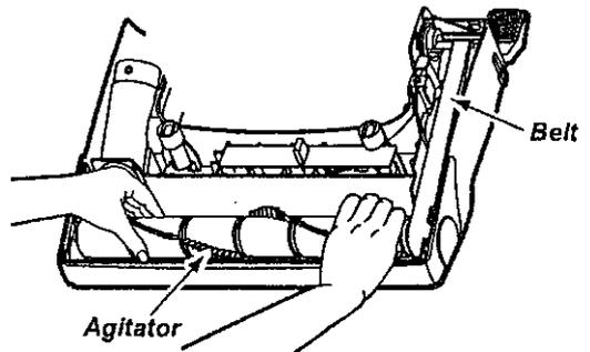
Position hands on the agitator. If the belt is still attached to the agitator, there will be tension on it.
