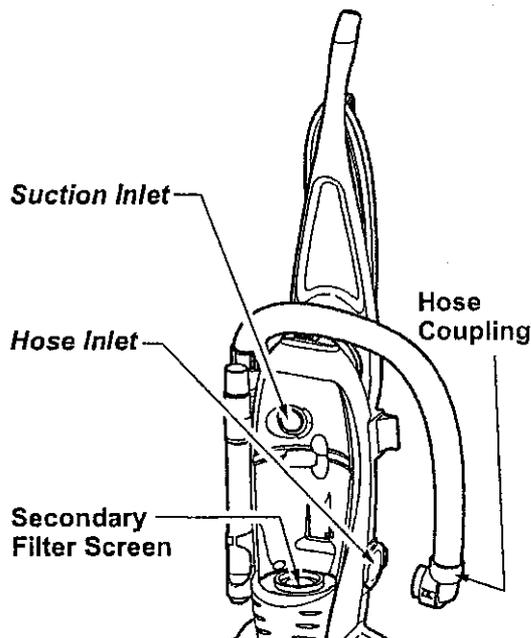
Unplug vacuum. Remove hose coupling and check hose coupling and hose inlet for clogs. Check suction inlet and secondary filter screen for clogs.
