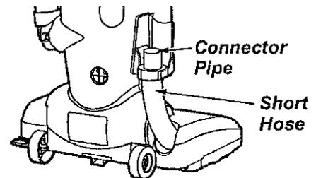
Disconnect wand from connector pipe and nozzle hose, check the wand and hose. Plug in vacuum cleaner and turn on.
