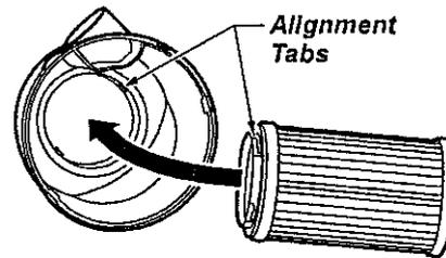
Rotate filter clockwise until slots lock onto tabs in lid.
