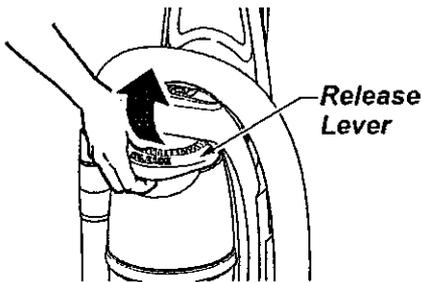
Remove dust bin from cleaner by tilting out as shown.
