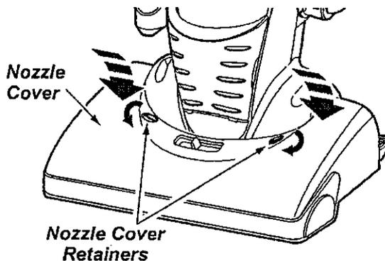
Make sure the nozzle cover retainers are in the UNLOCK position. Hook the front of the nozzle cover on to the nozzle base and rotate downward. Once in place, rotate the nozzle cover retainers to the LOCK position.
