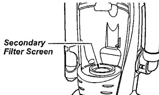
The secondary filter screen protects the motor.
