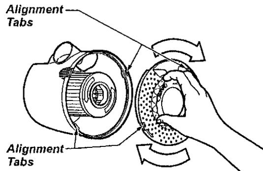
Rotate filter screen clockwise to lock in place.
