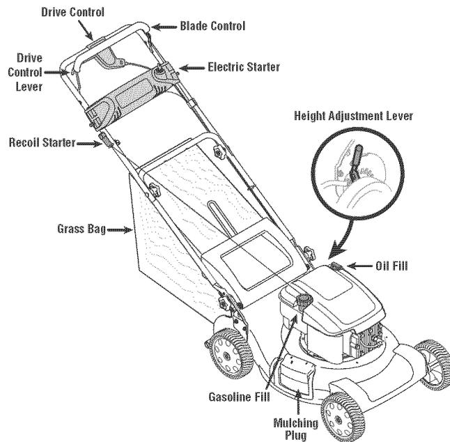
Figure 4-1: The major components on the mower.
