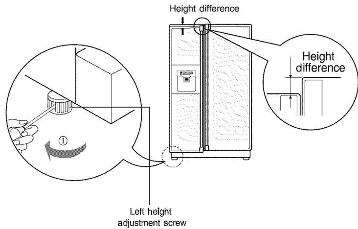
**If the freezer compartment door is higher than the refrigerator compartment door**
