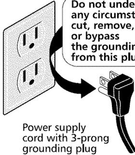
Power supply cord with 3-prong grounding plug
