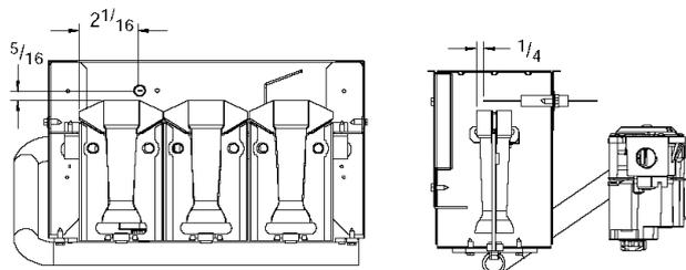
NOTE: Flame sensor has a different orientation in all 050 models.
