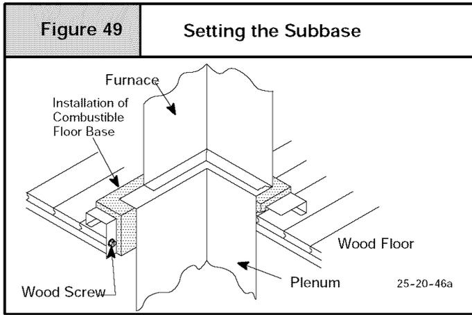
This subbase for combustible floors has been designed so that the height of the subbase raises the downflow coil off the floor to allow easy installation of the condensate drain. See **Figure 50**.
