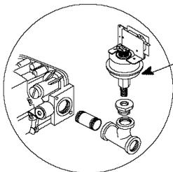
Drip Leg and Union, Union\* should be outside the cabinet. Manual shut-off valve MUST be upstream of dripleg, union, and furnace.
