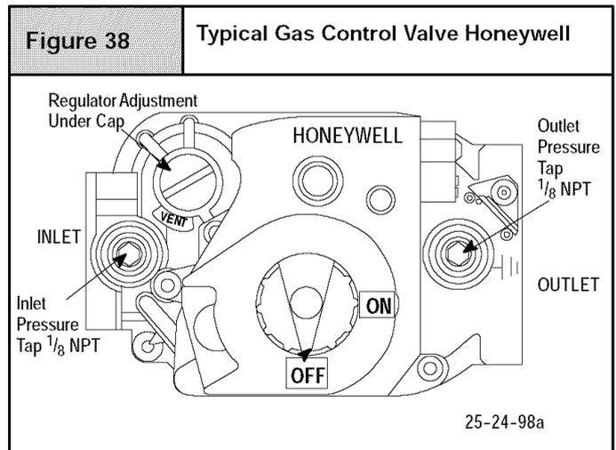
**NOTE:** Adjustment screw cover **MUST** be replaced on gas control valve before reading manifold pressure and operating furnace.
