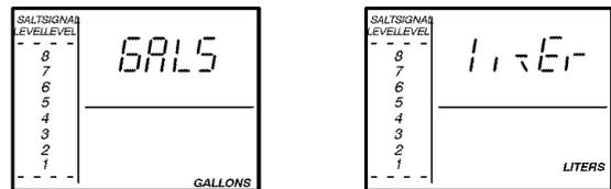
■ **Gallon or Liter readings:** Water usage and flow displays are shown in gallons. If you prefer to have the same displays in liters, press the UP button until Liter shows.
