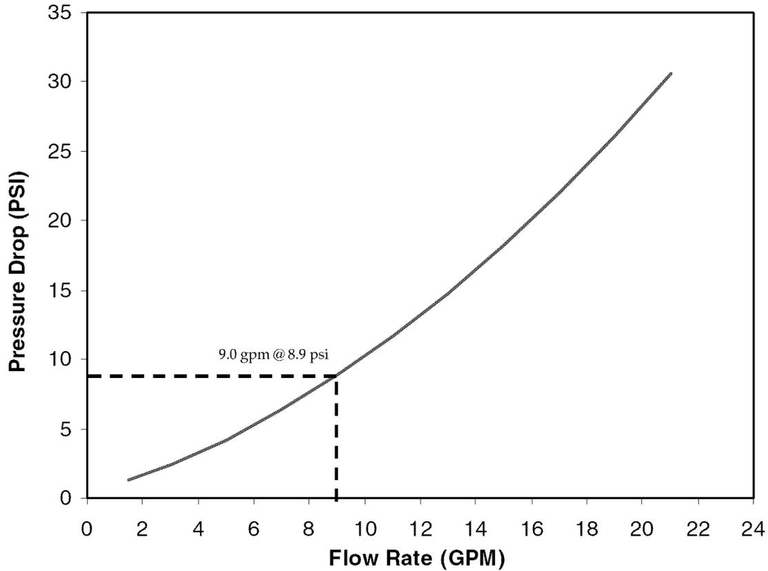
Intermittent flow rate does not represent the maximum service flow rate used for determining the softeners rated capacity and efficiency. Continuous operation at flow rates greater than the service flow rate may affect capacity and efficiency performance.
