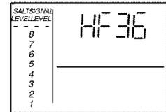
This code identifies the softener nominal capacity size. If the wrong number shows, the softener will operate on incorrect programming. Do the following as needed.
