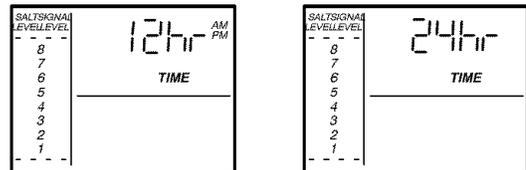
■ **12 or 24 hour clock:** All time displays are shown in standard clock time (1 to 12 PM; and 1 to 12 AM) at the 12 hr default setting. If military time displays are desired, set to 24 hr by pressing the UP button.
