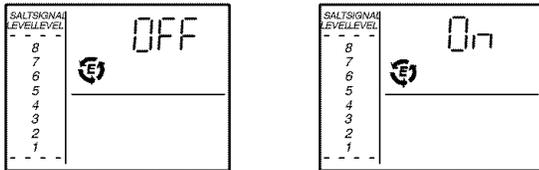
■ **SALT EFFICIENCY:** When this feature is ON, the unit will operate at salt efficiencies of 4000 grains of hardness per pound of salt or higher. (May recharge more often using smaller salt dosage and less water). For installations in the state of California, you must turn the Salt Efficiency Feature setting to ON.
