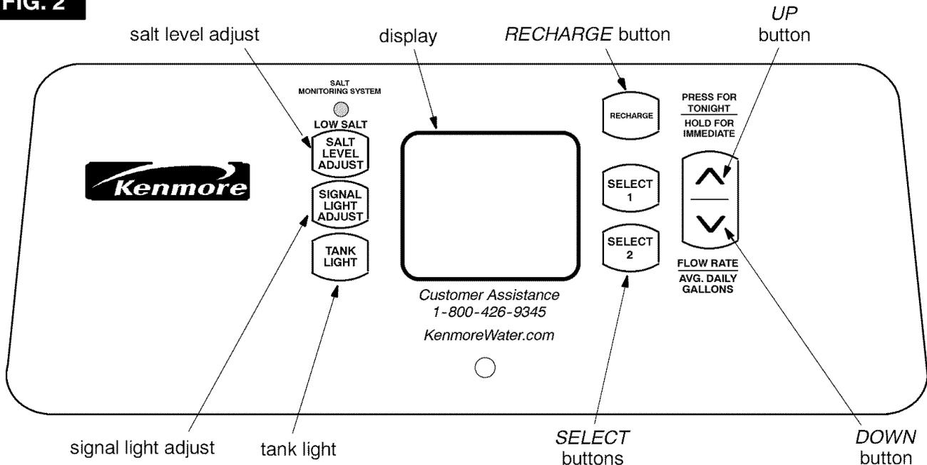
When the transformer is plugged in, the model code HF36, and a test number (example: J1.0) show in the face plate display for 4 seconds. Then, 12:00 AM and *PRESENT TIME* begin to flash.
