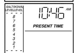
Each press of the UP /DOWN buttons changes the time by 1 minute. Holding the buttons in changes the time rapidly.
