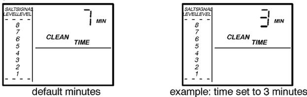
■ **CLEAN feature minutes:** If you are using this feature the length of the extra backwash cycle automat-
