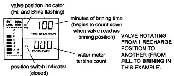
**POSITION SWITCH STATUS:** With the valve in service, or any of the recharge cycles, the switch indicator will show open  $\rightarrow$ . While the valve is rotating from one position to another, the indicator will show the switch closed  $\rightarrow$ . A defect is probable if indications vary from this pattern.
