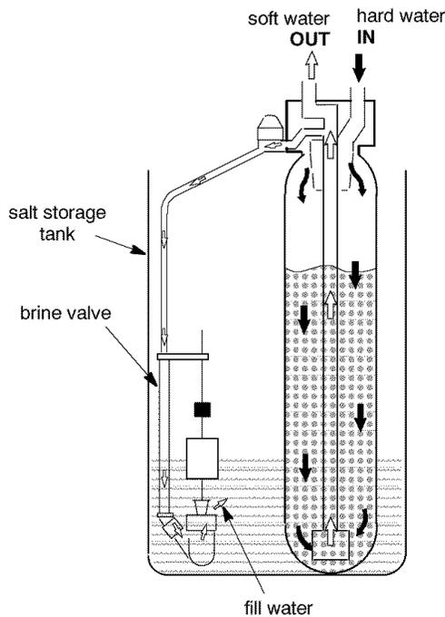
**2 BRINING:** During brining, the brine is moved from the salt storage area, into the resin tank. Inside the resin tank, brine cleans hardness minerals from the resin beads and they are discharged out the drain. How much brine is needed to clean the resin depends on:
