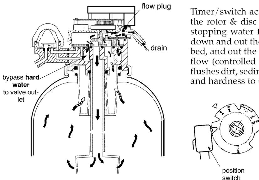
Timer/switch action again allows the motor to turn the rotor & disc to place the valve in BACKWASH, stopping water flow to the nozzle. Water is routed down and out the bottom distributor, up through the bed, and out the top distributor to the drain. The fast flow (controlled by a flow plug in the drain fitting) flushes dirt, sediments, iron deposits, remaining brine and hardness to the drain.
