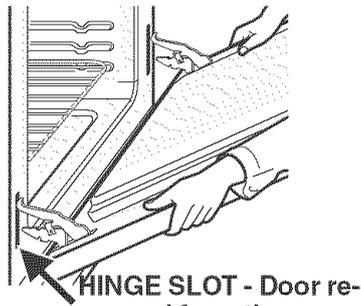
HINGE SLOT - Door removed from the oven
