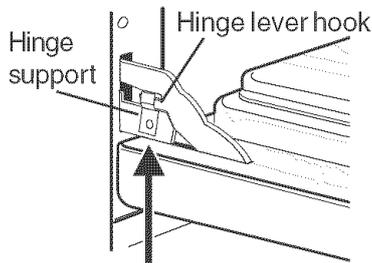
Lock engaged for door removal
