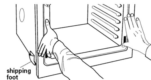
Push against seal area of front frame to push oven into cabinet until shipping feet almost contact cabinet. Use a Phillips screwdriver to remove screws attaching shipping feet. Remove and discard shipping feet.
