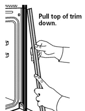
**3.** Remove trim screws attaching right and left side trim to oven. Grasp the bottom end of trim and pull away from oven. Slide top end of trim downward to remove trim from oven. Take care not to scratch other surfaces with ends of trim. Set trim and screws aside on protected surface.
