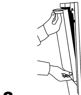
**2.** Completely open lower oven door. Insert small end of a door removal pin into each door hinge. Grasp door handle from the bottom and gently close door as far as it will shut. Lift slightly and grasp bottom of door with other hand. Pull door out at bottom to remove. Set door aside on protected surface. Repeat for upper oven door.
