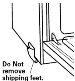
**1.** Turn power supply off. Move oven close to final position.
