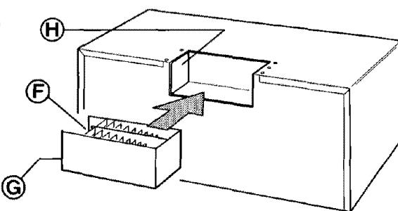
Slide air deflector back into cabinet as far as it will go. Check that deflector vanes ⑥ face the top of the cabinet and that the small exhaust ports ⑦ ⑧ face each other.
