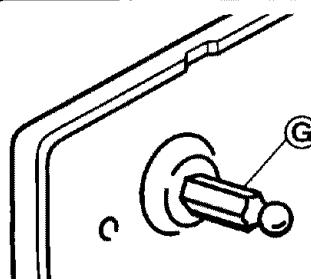
Rotate microwave hood up towards cabinet. Push microwave hood against mounting plate until locking pins **(G)** snap into cabinet.
