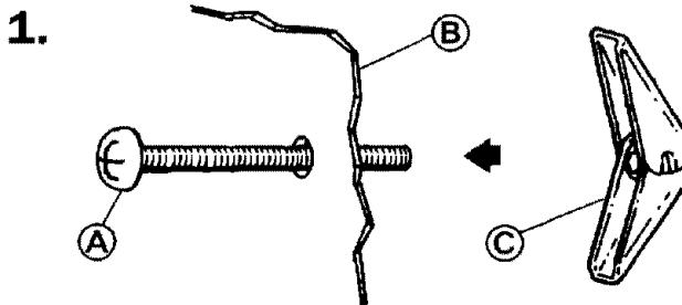
Insert 1/4" x 3" toggle bolts **A** through holes in mounting plate **B** that match the location of the 3/4" holes in the drywall.
