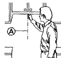
Using measuring tape, find and clearly mark the vertical centerline **A** of the cabinet opening on the wall directly under the upper cabinet.
