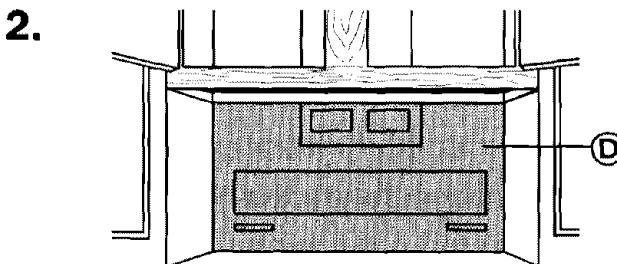
Position mounting plate **D** on the wall. Push toggle bolts **A** and nuts **C** through the drywall **E**.
