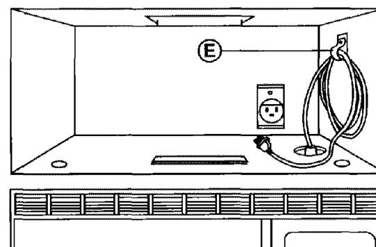
Coil power supply cord through clamp **E**. Secure clamp to cabinet side wall with dark colored screw.
