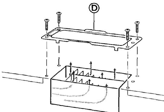
Reattach damper plate ⑤ with four screws at each corner of the damper plate. Save bright-colored tapping screw for use later to attach damper assembly.
