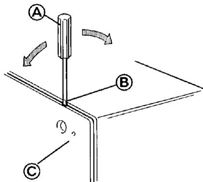
Loosen tape to open door. Do Not remove tape.
