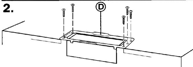
Remove 5 screws that attach damper plate **D** to top of microwave hood cabinet.
