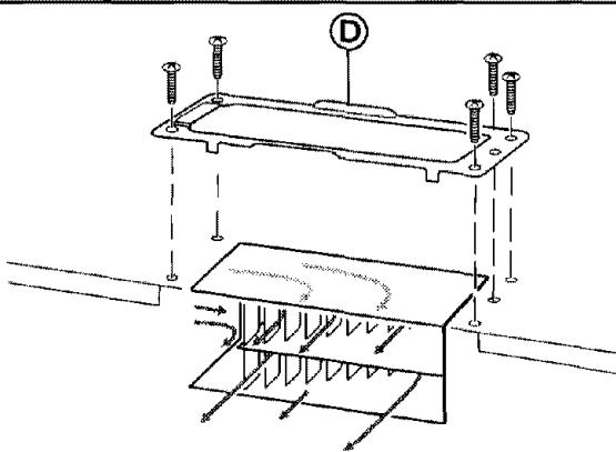
Reattach damper plate ⑤ with five screws.
