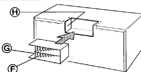
Slide air deflector back into cabinet as far as it will go. Check that deflector vanes **F** face the rear of the cabinet and that the small exhaust ports **G** **H** face each other.
