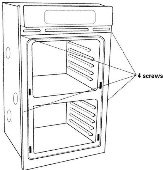
**6.** Important: Securely fasten oven to cabinet using the screws provided (two screws for a single oven or four screws for a double oven). Insert the screws through holes in mounting rails. Do Not overtighten screws.
