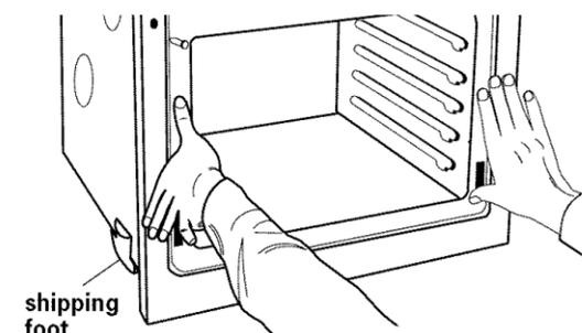
Push against seal area of front frame to push oven into cabinet until shipping feet almost contact cabinet. Use a Phillips screwdriver to remove screws attaching shipping feet. Remove and discard shipping feet.
