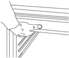
**5.** Lift oven into cabinet cutout using the oven opening as an area to grip.
