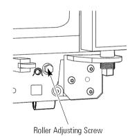
• Use a 3/8" hex socket or wrench to turn the adjustment screws. Turn the screws clockwise to raise the refrigerator, turn counterclockwise to lower it.
