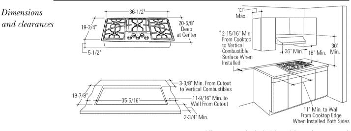
\* If a countertop backsplash is used, it must be constructed of non-combustible materials (such as masonry, ceramic, granite, stainless steel, etc.) whenever the cutout to rear vertical surface is less than 3-3/8".
