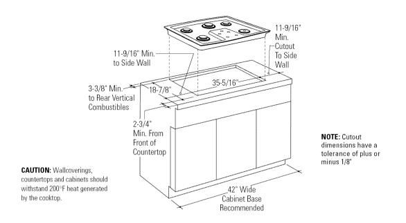
Measure carefully when cutting countertop. Make sure sides of opening are parallel and rear and front cuts are exactly perpendicular to sides.
