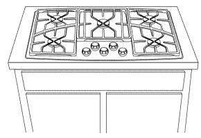
These models are factory set for either natural gas or LP gas operation. Be sure to order the correct model for the installation situation.
