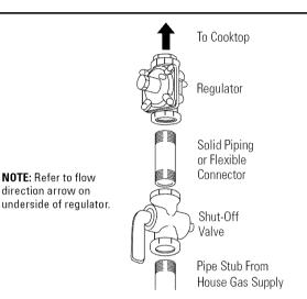
**IMPORTANT:** Disconnect the cooktop and the individual shut-off valve from the gas supply piping system during any pressure testing of that system at test pressures greater than 1/2 psig. Isolate the cooktop from the gas supply piping system by closing the individual manual shut-off valve to the cooktop during any pressure testing of the gas supply piping system at test pressures equal to or less than 1/2 psig.
