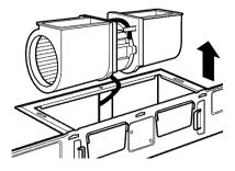
**6** Roll the blower unit 90° so that fan blade openings are facing toward the front of the microwave.
