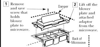
3 Slide exhaust adaptor to one side and remove it. **NOTE:** The exhaust adaptor with damper is not needed for recirculating models. You may want to save them for possible future use.
