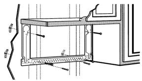
Attach the plate to the wall using toggle bolts. At least one wood screw must be used to attach the plate to a wall stud.
