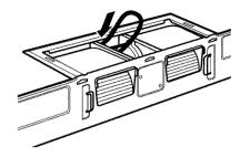
8 Secure the blower unit to the microwave with the screw from Step 1.
