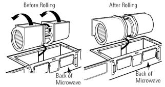
4 Gently slip the wire through the gap between the two tabs on the top of the blower so the wire is behind the tabs.
