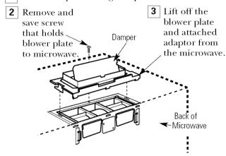
**4** Slide exhaust adaptor to one side and remove it.
