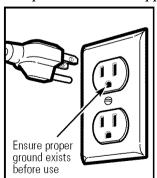
three-prong (grounding) plug which mates with a standard three-prong (grounding) wall receptacle to minimize the possibility of electric shock hazard from this appliance. You should have the wall receptacle and circuit checked by a qualified electrician to make sure the receptacle is properly grounded.
