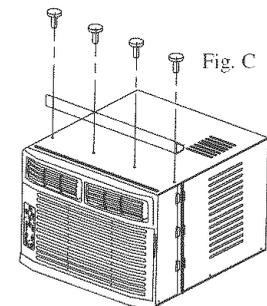
D. Secure the top rail to the unit with the 3/8" Screws as shown in Fig. C
