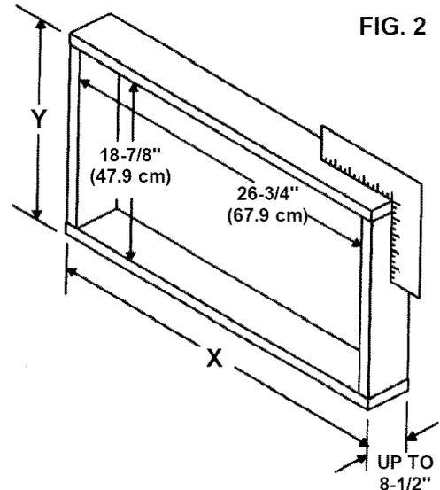
4. Build a wooden sleeve with the INSIDE dimensions of 26-3/4" (67.9cm) in width and 18-7/8" (47.9cm) in height. Frame depth should be the same as wall thickness. Fill in the space from the opening to the studs with wood spacers, as shown.
