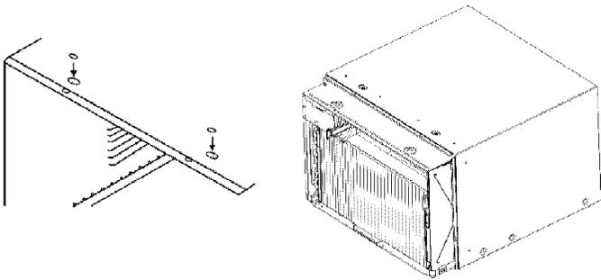
2. Before proceeding to STEP 2 add the two (2) short seals to cover the holes where retaining screws were.
