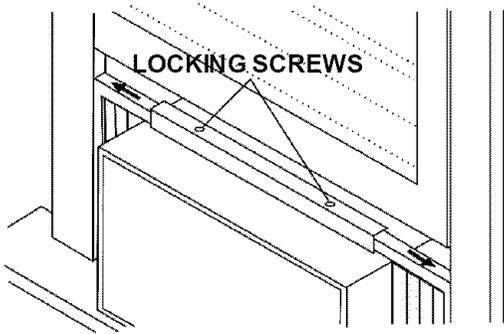
2. Extend panels to fill window opening completely. Tighten locking screws on top.
