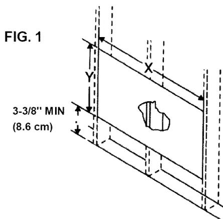
Carefully measure and cut an opening with the following dimensions. See FIGS. 1 and 2.
