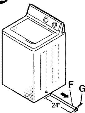
Move washer close to final position. Make sure there is at least a 24" clearance on right side of washer to remove shipping bar F. **PULL SHIPPING BAR F OUT USING YELLOW PLASTIC HANDLE G.** Keep bar so it can be reinstalled if washer is ever moved again.
