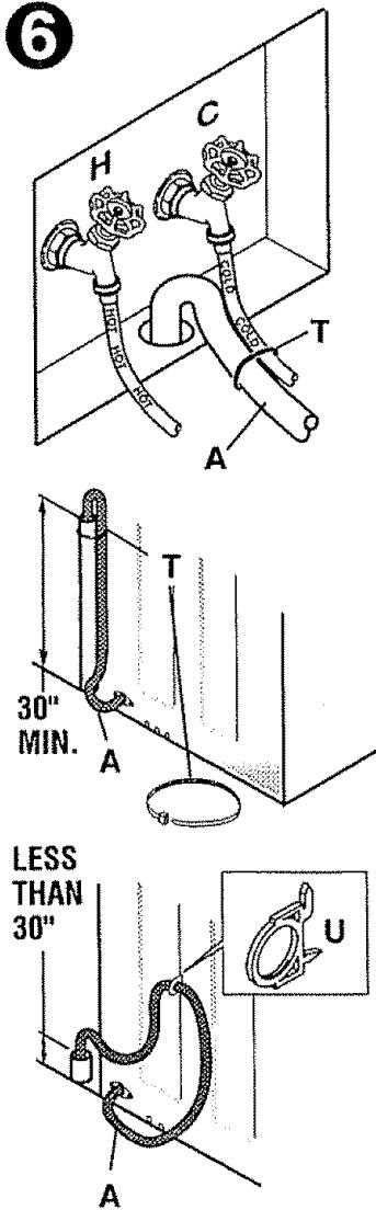
**NOTE:** If longer drain hose is required, order drain hose extension kit, GE part number WH49X301. Connect additional drain hose (contained in kit) to original hose with hose clamp (contained in kit).
