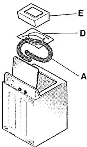
After the machine is in the home, remove remaining packing material/carton from washer.
