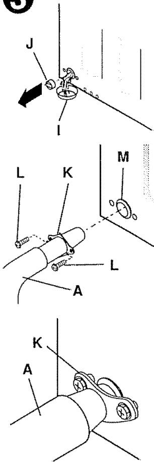
Place a cooking dish or pan **I** under drain opening on back of washer. Pull plug **J** out of grommet **M** with pliers and discard. Water left over from factory test will drain. Remove container **I** and water.
