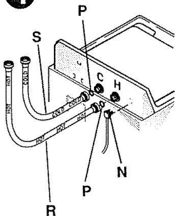
Remove electrical cord **N** from storage before installing water hoses. Install rubber washer **P** in one end of hot water hose **R**. Thread hot water hose **R** onto connection labeled **H** at top rear of washer. Hand tighten, plus an additional 1/8 turn with pliers.
