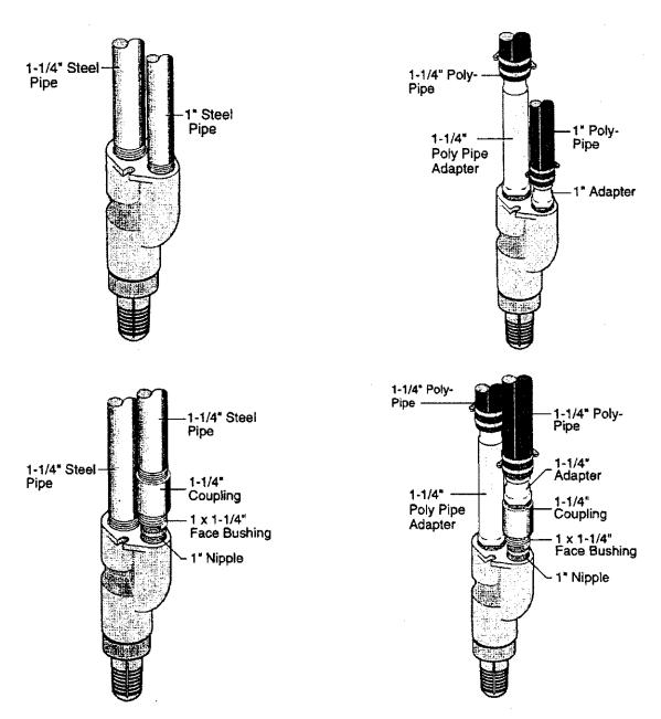
IMPORTANT: Use pipe thread compound on male threads and tighten Venturi Adapter or Steel Pipe Into Jet Body.
