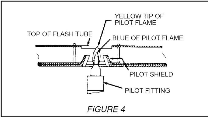
Purge all air from supply system by turning on one top burner valve. Then turn off valve and adjust top pilot flame using pilot adjusting screw (figure 5) so that flame is even with top of flash tube. See figure 4. To light the burner, push and turn top burner knob to the lite position.
