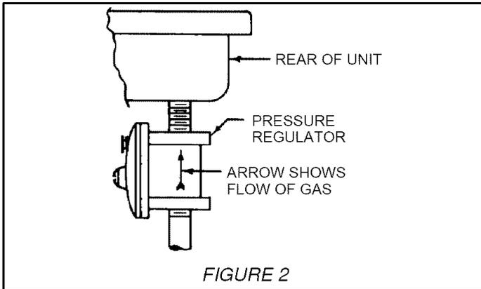
The gas appliance pressure regulator for the top section (see figure 2) is located in the pack out box for shipment. The burner orifices, etc., are sized for the gas pressure delivered by the regulator supplied - IT MUST BE INSTALLED before operating the top section. For convenience of service, it should be installed as shown in figure 2. The regulator must be accessible for adjustment after installation.
