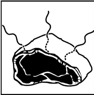
The microwaves disturb water molecules in the food. As the molecules bounce around bumping into each other, heat is made, like rubbing your hands together. This is the heat that does the cooking.
