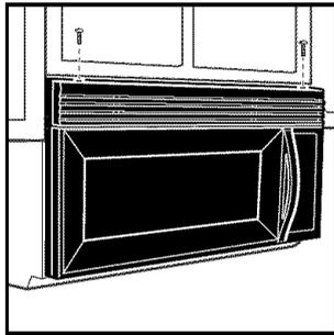
3. Tip the grille forward, then lift out to remove.
