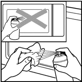
**NOTE: Abrasive cleansers, steel-wool pads, gritty wash cloths, some paper towels, etc., can damage the control panel and the interior and exterior oven surfaces.**
