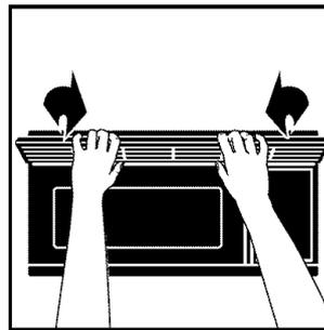
Push the bottom until it snaps into place. Replace the mounting screws.
