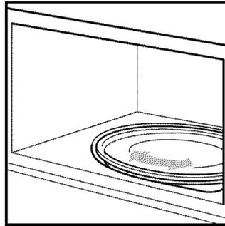
**Make sure** the rollers are completely inside the center circle of the turntable; this will let the turntable rotate properly.
