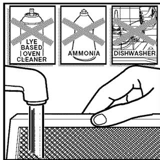
**Do not use ammonia, corrosive cleaning agents such as lye-based oven cleaners, or place in a dishwasher. The filter will turn black or could be damaged.**
