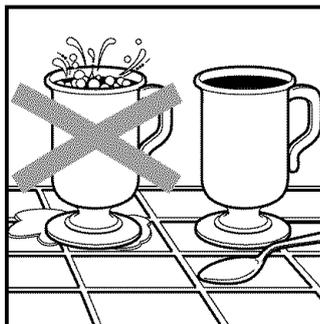
Liquids heated in certain containers (especially containers shaped like cylinders) may become overheated. The liquid may splash out with a loud noise during or after heating or when adding ingredients
