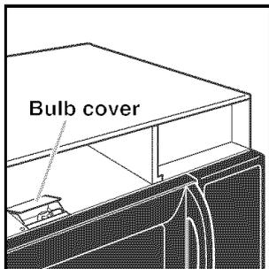
5. Replace the bulb with a candelabra-base 30-watt bulb (PN 4393681).†
