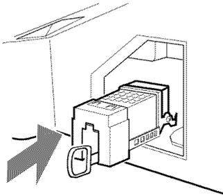
**⚠** If the lamp is not securely reattached, the self-diagnostic function may be triggered and the POWER/STANDBY indicator flashes three times (see page 12).
