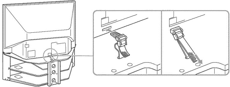
**When using the SU-RG11S (for KDF-E42A10)/SU-RG11M (for KDF-E50A10) stand for your TV, you must use the support belt.**
