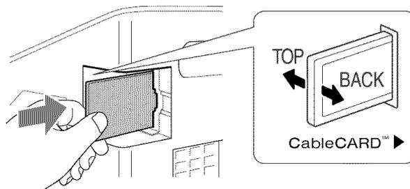
**CAUTION:** When inserting the CableCARD device, the rear side of the card should face forward. Inserting the CableCARD incorrectly may result in permanent damage to the card and the TV.
