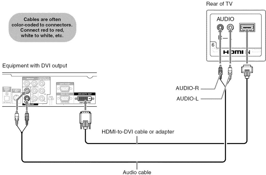
**When using a HDMI-to-DVI cable or an adapter, be sure to connect the DVI output connector first; then connect to the HDMI input on your TV.**
