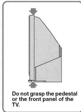
When moving the TV, place one hand in the hole on the lower portion of the TV while grasping the top with the other hand, as shown in the illustration below.
