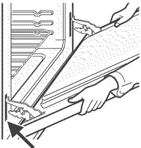
HINGE SLOT - Door removed
