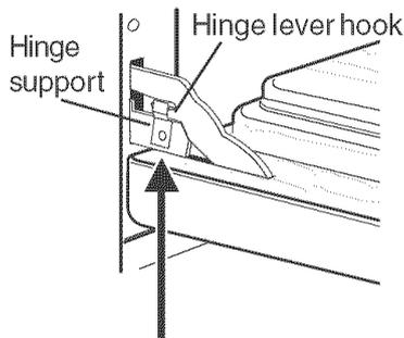
Lock engaged for door removal
