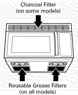
The vent fan has 2 metal reusable grease filters.
