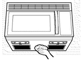
Clean off the grease and dust on the bottom often. Use a solution of warm water and detergent.
