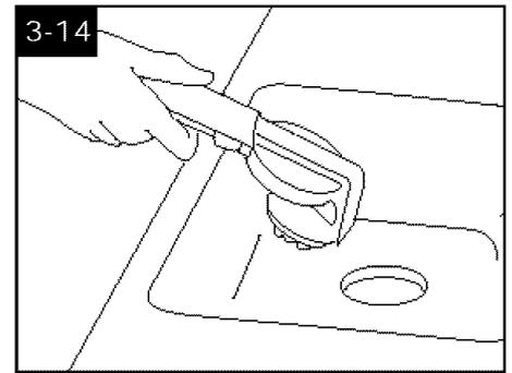
3. Drain hose by turning deep cleaner ON and holding end of hose up for several seconds. Do not press trigger.
