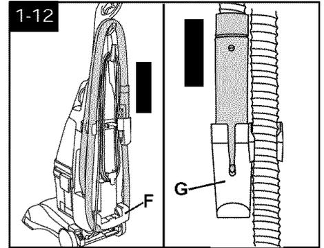
Continue wrapping hose under lower hook (F). Snap hose end **fully** into holder (G).
