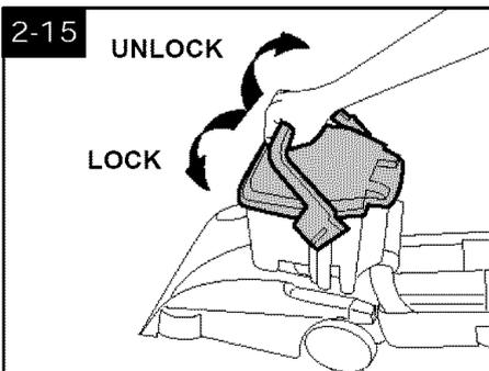
Raise handle to carrying position (straight up) to **unlock tank** from base of deep cleaner. Lift tank from deep cleaner and carry it to a sink or drain.
