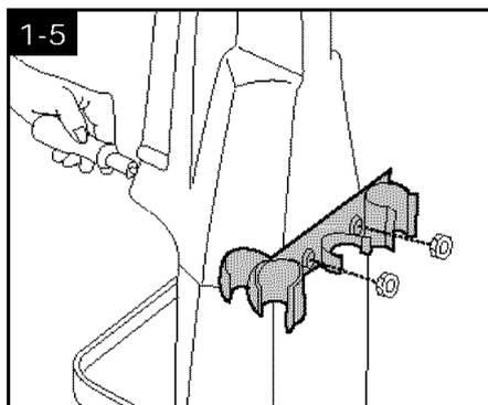
Place **nuts** in recessed areas on **back of handle**. Hold each nut in place while tightening each bolt securely (from the front of the handle) with a Phillips screw driver.
