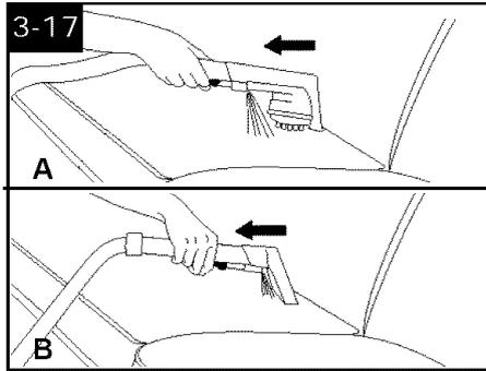
Press the trigger and slowly pull the nozzle over the fabric.
