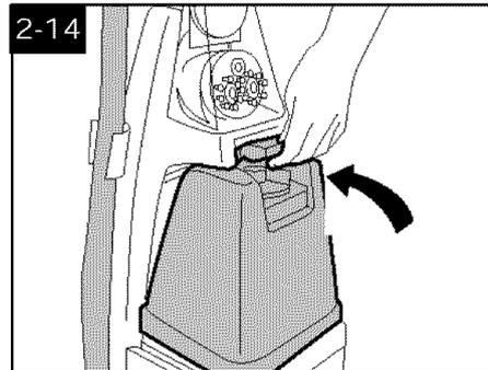
Position bottom of tank into unit and press on tank handle to snap tank into place.
