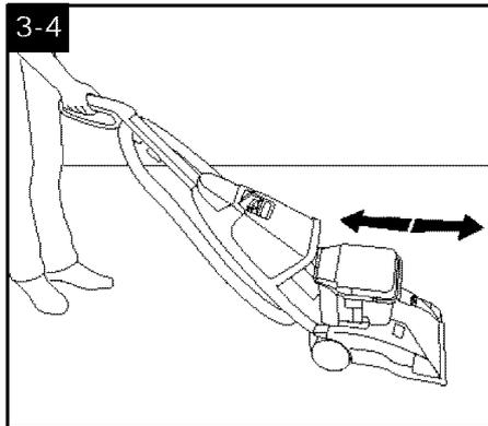
5. Squeeze trigger to release cleaning solution and **slowly** push deep cleaner forward (equals one wet stroke).
