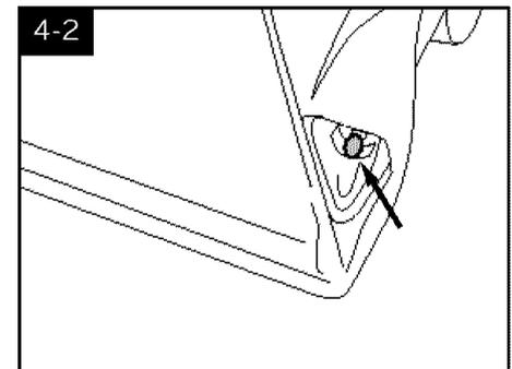
2. Pull old bulb straight out of socket.
