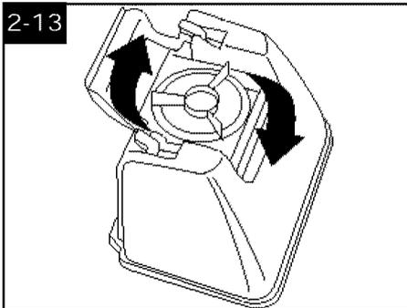
Replace cap. **Rotate cap clockwise until it locks in place. Cap must be locked in place for proper performance and to prevent leaking.**
