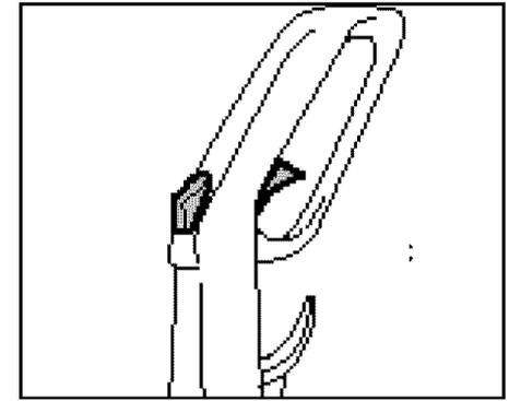
When handle sections are completely together, squeeze trigger (C) and depress Clean Surge™ Button\* (D) on upper handle.
