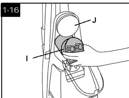
To remove powered hand tool (I), pull it down and outward.
