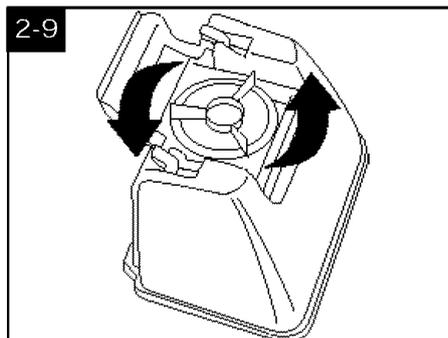
Carry tank to a sink. Rotate tank cap counterclockwise and lift up to remove cap.
