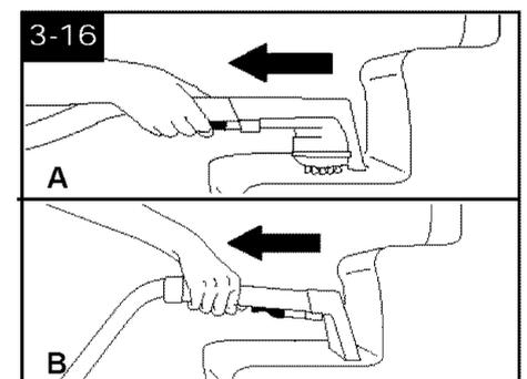
9. Lift tool, and position it against riser. Pull tool **slowly** over carpet without pressing trigger (dry stroke).
