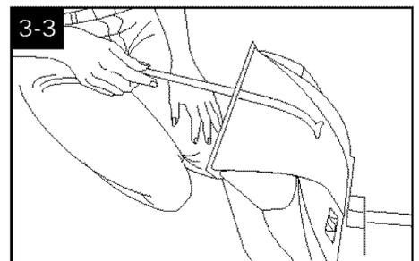
**Some models have a nozzle clean-out tool** for removing debris or if a non-carpeted floor is not available. To use the tool:
