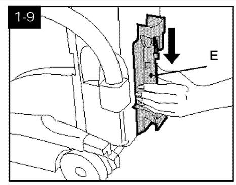
Slide rack down into place. Insert screw at (E) and tighten with a Phillips screwdriver.
