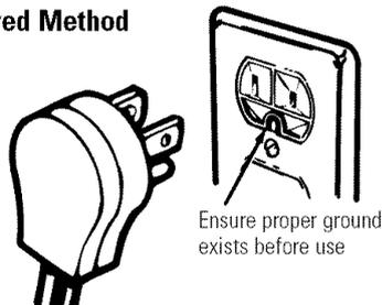
The power cord of this appliance is equipped with a three-prong (grounding) plug which mates with a standard three-prong grounding wall receptacle to minimize the possibility of electric shock hazard from this appliance.
