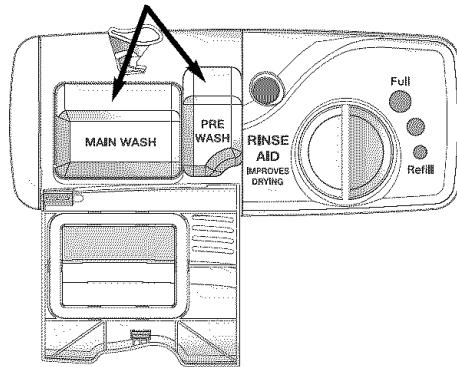
Do not use detergent with the Rinse Only (select models) cycle. Leave the detergent lid open when running Rinse Only (select models).
