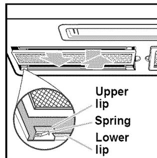
4. This model comes with Dishwasher Safe Grease Filters. Place the grease filters in an empty dishwasher and wash. **NOTE:** Washing these filters with dirty dishes may cause the filters to trap the particles from the dishes, so we recommend washing separately in an empty dishwasher.
