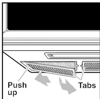
3. To remove the charcoal filters, push the back of each filter away from you. This will slide the front of the filter off the lower lip. Swing the front of the filter down and slide the filter out.
