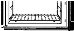
**Bottom position:** Insert rack securely on bottom of oven when using taller containers.
