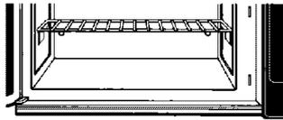
**Normal position:** Insert the rack securely on the rack guides on the side walls of the oven.
