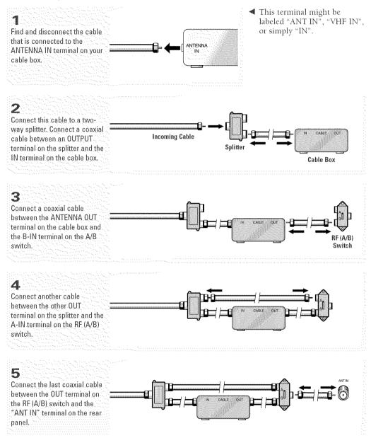
After you've made this connection, set the A/B switch to the "A" position for normal viewing. Set the A/B switch to the "B" position to view scrambled channels. (When you set the A/B switch to "B," you will need to tune your TV to the cable box's output channel, which is usually channel 3 or 4.)
