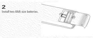
■ Make sure to match the "+" and "—" ends of the batteries with the diagram inside the compartment.
