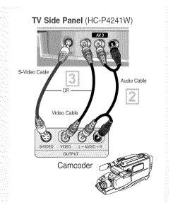
This figure shows the Standard connector-jack panel. The actual configuration for your TV may be different.
