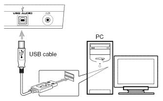
· Use "USB series A plug to B plug" cable when connecting.
