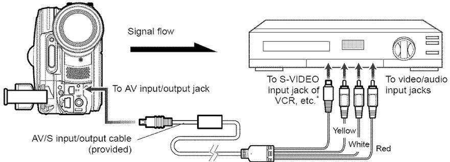
\* If the video device to be connected has an S-VIDEO input jack, you can connect it to the DVD video camera/recorder.
