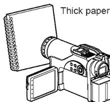
If focus is not correct when the white object fills the screen, manually focus the object, referring to "Manually Focusing Subject" (see page 72).
