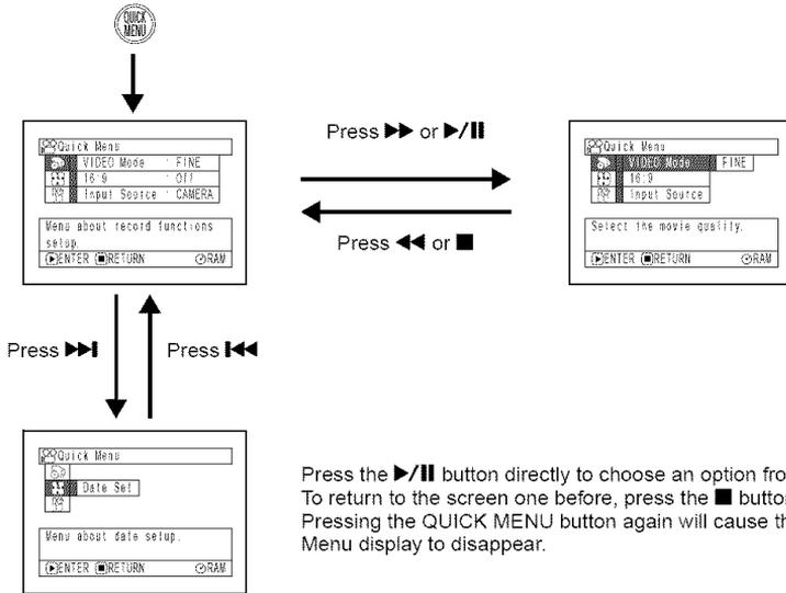
Press the **▶/||** button directly to choose an option from menu. To return to the screen one before, press the **■** button. Pressing the QUICK MENU button again will cause the Quick Menu display to disappear.
