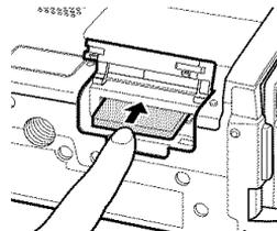
④ Insert the card all the way until it locks, and then close the cover of card insertion block.
