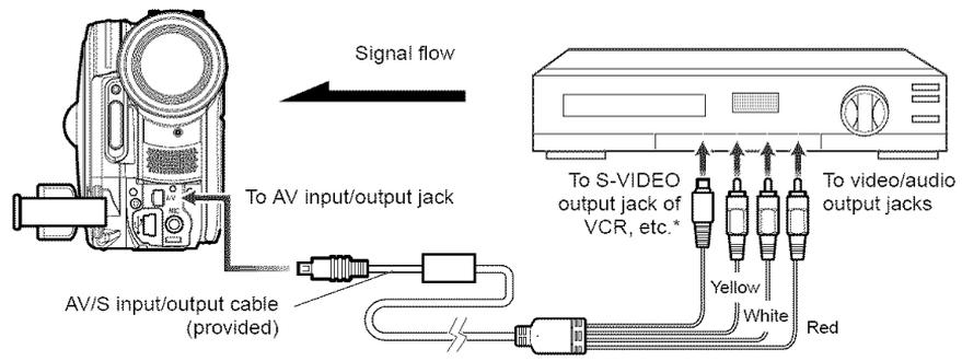
\* If you are using DZ-GX20A or DZ-MV780A, and the connected AV device has an S-VIDEO output jack, you can connect the S-VIDEO jack of AV/S input/output cable.
