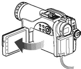
② While holding down the button on the right of power switch, set the switch to "V" or "M" (only "V" for DVD-R disc).
