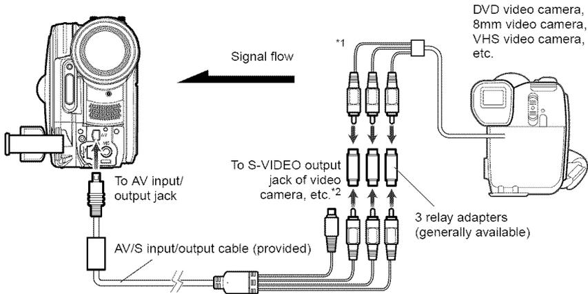
\*1: The AV/S input/output cable provided with this DVD video camera/recorder can be directly connected to some video cameras.
