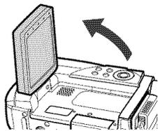
② Open the cover of card insertion block with power turned off.
