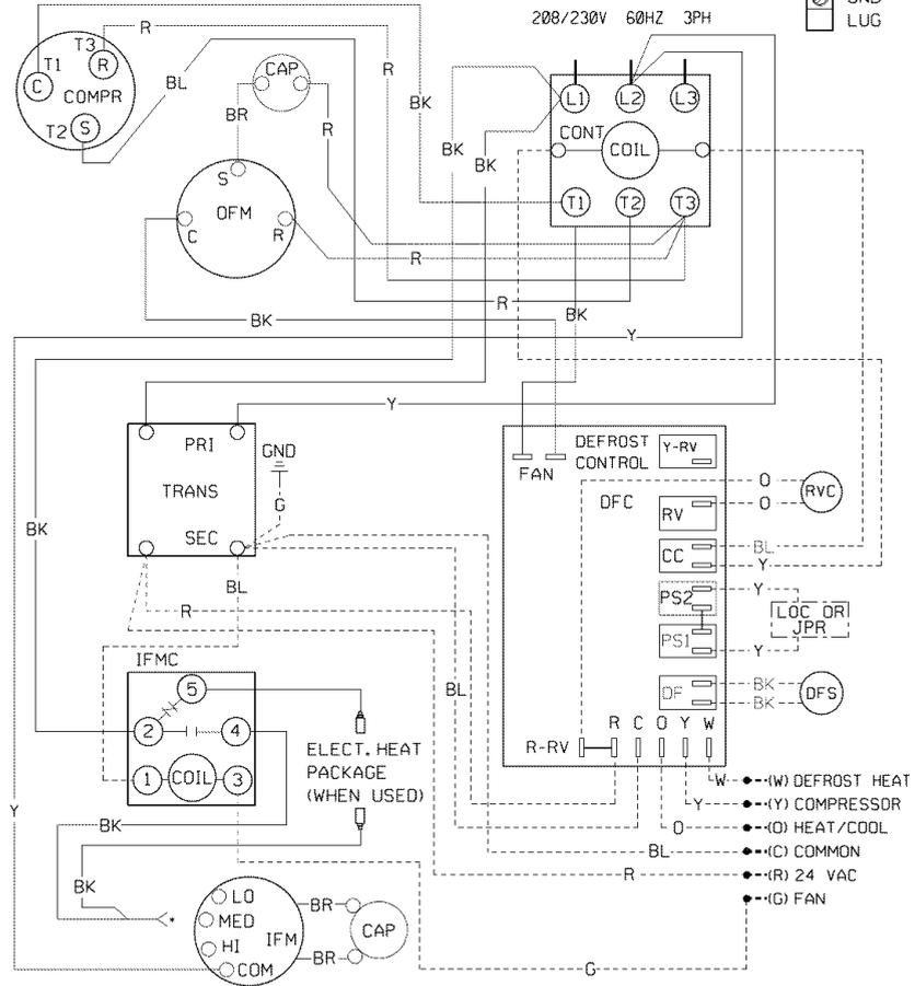
IF ANY OF THE ORIGINAL WIRE AS SUPPLIED WITH THE APPLIANCE MUST BE REPLACED, IT MUST BE REPLACED WITH TYPE AWM-105°C OR ITS EQUIVALENT,
