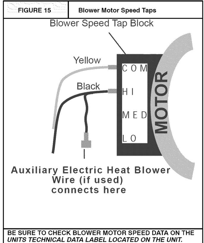
**NOTE:** On Heat Pumps Electric heater blower wire must be attached to the same speed tap required for cooling/heat pump operation. **See FIGURE 11 notes.** The **yellow** lead **MUST** always be connected to the speed tap block at the common quick connect terminal. The terminal is identified as **COM**.
