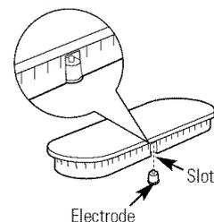
Make sure the slot in the burner head is positioned over the electrode.
