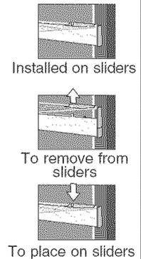
Pull oven rack forward and lift it up off the oven rack slider.
