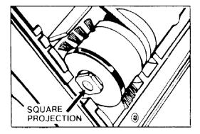
8. Reposition agitator by sliding square projection on belt end of agitator into square slot on side of nozzle. Then slide round projection on other end of agitator into round slot. Note: Be sure ribs on agitator fit outside ribs in cleaner as shown.
