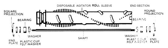
5. Replace parts onto new agitator roll sleeve.
