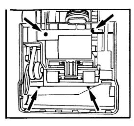
Remove the four hood mounting screws, as shown.
