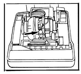
Turn cleaner over, pull up on nozzle control knob to disengage; and lift up hood. Pull out old bulb and push in a new one.
