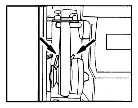
Be sure lower edges of belt are positioned between sides of wire guide.
