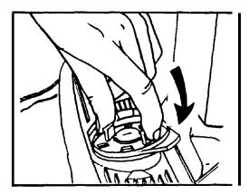
Replace cover, aligning center opening with shaft and lock by turning clockwise.
