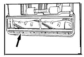
Replace bottom plate by fitting front edge under tabs on front of nozzle. Insert screws and tighten.
