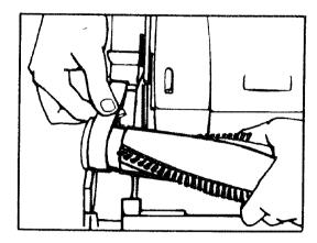
6. Place one end of the new belt over the metal motor pulley. Lettering on belt should be visible and not against pulleys. Slip the other end around the plastic pulley end of the agitator. (See illustration)
