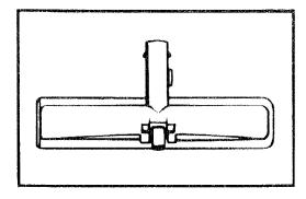
The converter must first be assembled to the hose by inserting the converter into the hose connector.
