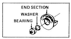
5. Should you accidentally displace the bearing during disassembly, reassemble as shown. Replace belt, agitator and bottom plate.
