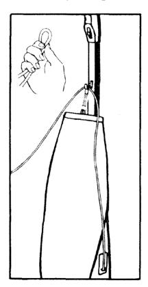
Make a small loop with cord and place it over the hook at the back of the handle. When operating, cord should be positioned as shown.
