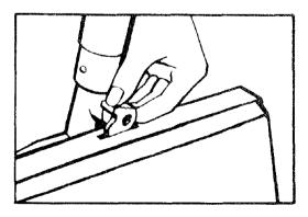
Place edge of lock in slot on cleaner and turn lock to secure converter.
