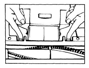
13. Lift and snap retaining clips into place.
