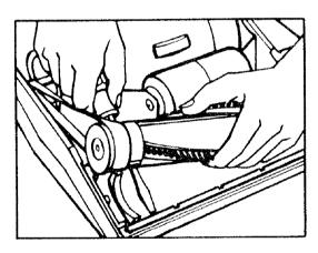
4. Use one hand to remove the agitator as you use leverage to lift the agitator with the end of the screwdriver. Remove old belt.
