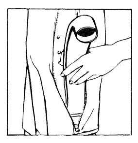
Remove paper bag from inside the vinyl jacket. Then remove dirt tube by pushing to either side to release retention clips. Lift tube up and out.
