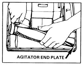
7. Grasp the agitator frimly with one hand. (Be sure you can see the agitator end plate.) Engage screwdriver as shown for leverage.
