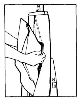
3. Push cardboard bag collar firmly onto fill tube by first, positioning bottom of collar, and then top, onto tube. Make sure the collar is pushed past the raised portion at the top and bottom and tightly in place on the tapered portion of the tube. This will insure a firmly sealed position.
