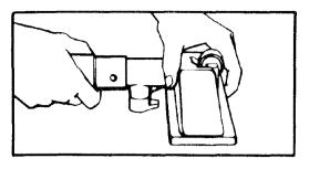
Push connector and converter together and twist until the projections on the converter fit into the holes on the hose connector. This unit should remain assembled for all future tool use.
