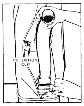
For access to the dirt tube, first remove disposable bag. Then remove dirt tube by pushing to either side to release clips. Lift dirt tube up and out.
