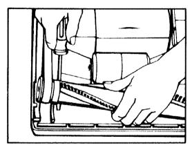
8. Lift and pull using screwdriver as a lever. Guide the end opposite the belt into position first.
