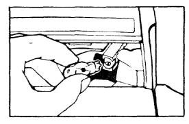
4. Remove bulbs by pulling straight out of sockets. Replace by pushing each bulb straight into the socket until it locks in place. (Excessive force is not required).
