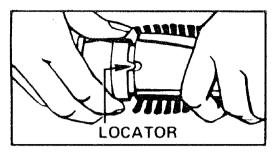
4. Reassemble agitator parts. Line up locator on end sections with slot on agitator. **Note:** Large locator on pulley end must align with large notch on agitator.
