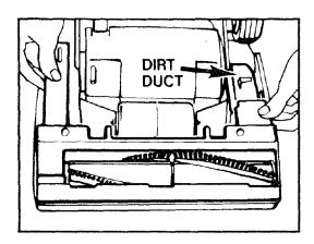
12. Maintaining front connection, rotate bottom plate to cover bottom of cleaner. Make sure dirt duct is in position under bottom plate. Press firmly.
