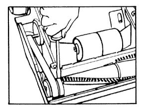
3. To remove the agitator, use a screwdriver placed as shown.
