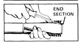
2. Pull or pry out end sections as shown in illustration.
