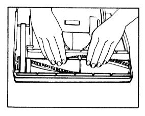
10. Press firmly to be sure agitator is securely in place.
