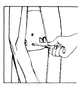
Insert the two screws into the holes provided inside the front housing.
