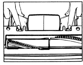
1. Turn cleaner over. Release handle to lowest position. Remove plate on bottom of cleaner by releasing clips. (See illustration)
