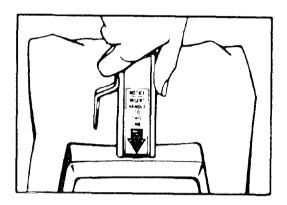
Insert handle into the cleaner to the line indicated on label. Insertion to the line is necessary for proper screw alignment.
