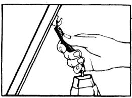
Lower handle to operating position and place spring bag ring over hook located on handle.
