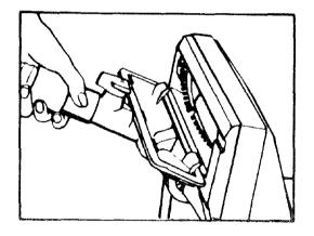
Place projections on converter onto rim on bottom plate of cleaner.
