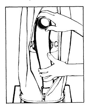
To replace dirt tube, position over lower seal and push down. Insert one side against retention clips. Push to snap other side into position.
