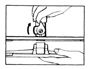
Turn lock on converter so that the serrated portion is in line with the hose.
