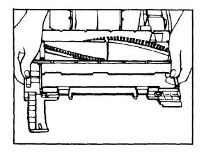
11. Bottom plate attaches in a hinge-like motion. Place the groove on the front of the bottom plate over the notched edge on the front of the cleaner.
