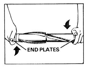
5. If the end plates have loosened, tighten them by turning in opposite directions.
