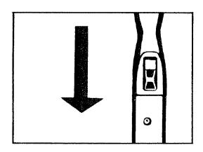
Turn the plastic ring as shown to lock the tool in place. To remove tools, reverse the procedure.
