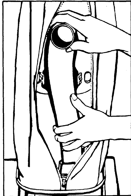
To replace dirt tube, position over lower seal and push down. Insert one side against retention clips. Push to snap other side into position.
