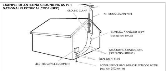
Note to the CATV system installer: this reminder is provided to call the CATV system installer's attention to Article 820-40 of the NEC that provides guidelines for proper grounding and, in particular, specifies that the cable ground shall be connected to the grounding system of the building, as close to the point of cable entry as practical.
