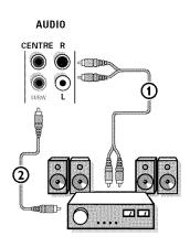
Connect the audio cable to the multi channel Surround receiver and to AUDIO RECEIVER L and R next to the CENTRE connector of your TV 1.
