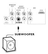
To enhance the sound reproduction of your TV you can connect an externally powered subwoofer (between 20 and 250 Hz).
